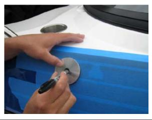
Once the desired position is achieved, place one of the large nylon whasers over the piece of tape and trace around it with a permanent marker.
