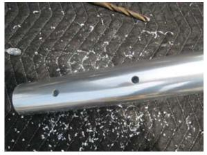
Use a smaller bit to make a pilot hole, then use your 27/64" bit.
