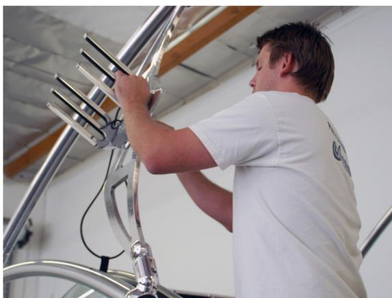
To install the board rack fingers, use the socket head cap screws provided and attach the fingers to the diamond shaped plate. This diamond plate will then be installed to the rear switch blade legs.
