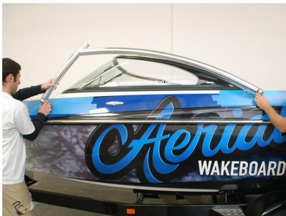
Once the feet are connected to the side rails, hold the side rail up to your boat. Once the rail is aligned with your windshield use a small piece of tape to mark the position of the mounting feet.
