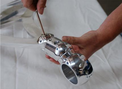
The lower section of the switch blade can now be assembled to the lower fittings and clamp using the trim washer, M12 X 45mm socket head cap bolt and threaded lap joint.
