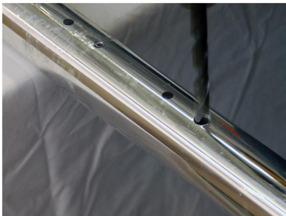
Following the pilot holes you just drilled, use a 27/64" drill bit to create the clearance hole for the joining bolts.
