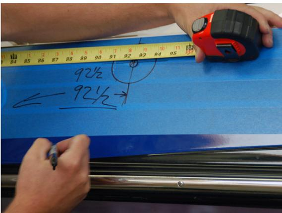
It is best to take measurements from the back of the boat and mark with blue tape. Be sure to measure from the same point on both sides.
