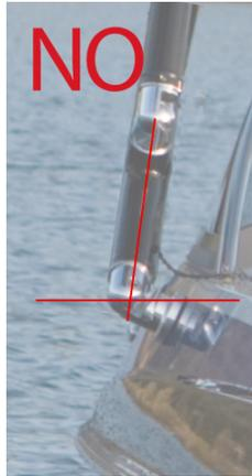
The side rails need to be mounted straight up and down. If they are leaning in or out, this will cause a problem with the tower when you want to fold it.
