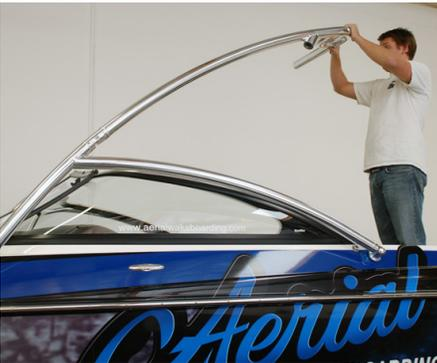
Insert the front leg hinge joint into the lower section of the front arm (repeat for the other side). Its important not to completely tighten the fittings as some adjustment will necessary before the installation is complete.
