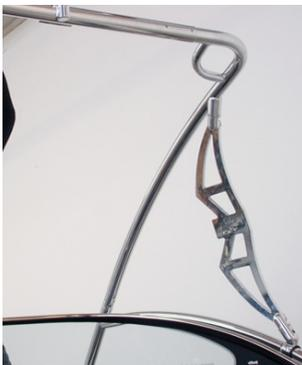
The rear switch blades can now be installed by attaching the top switch blade fitting to the fitting located on the upper section of the front leg. The clamp located on the base of the switch blade will be connected to the lower side rail. We recommend making sure that the clamps on both sides of the tower are located the same distance from the end of the side rail so that your tower looks symmetrical.
