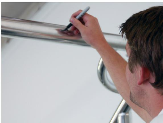
Using the pre-drilled holes in the top section tube, mark the drilling positions on the front leg tubes. Before making your marks, check to ensure that the tow point is aligned correctly and positioned vertically. The tow point should also be positioned on the rear of the top section tube so that the logo plate is facing towards the bow of the boat.
