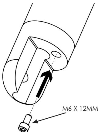
Once you are happy with your tower installation and all of the fittings are lined up to allow the tower to fold and function correctly it will then be important to firmly lock the fittings in place to prevent any unwanted rotation or loosening. We recommend using threadlocker during this step.
