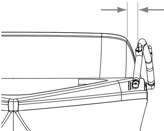
Measuring from your windshield, check the distance to the side rail to make sure both sides are symmetric.
