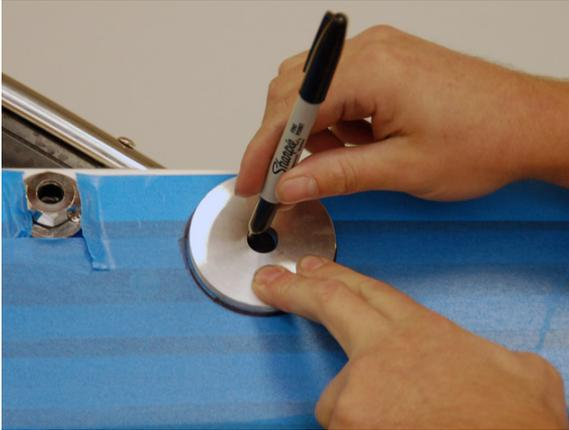
Once the desired position is achieved, place one of the nylon mount washers over the piece of tape and trace around it with a permanent marker.
