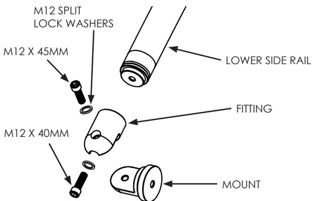
The mounting feet will need to be assembled to the side rail fittings, followed by attaching them to the side rails.
