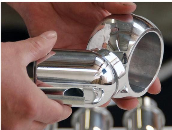
You will then need to attach the lower base to the threaded lap joint. This is then followed by attaching the clamp to the lower base (using the stainless steel socket head cap screw.)
